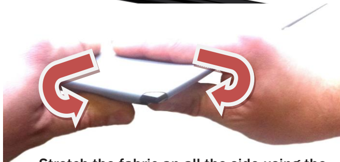
Stretch the fabric on all the side using the rod profile.
