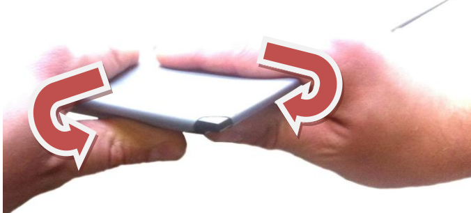
Stretch the fabric an all the side using the rod profile.
